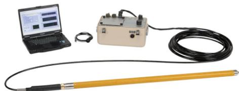
Dart packs the power of magnetic resonance logging into a highly portable, battery-powered system operable by a single user. With Dart, any small-diameter bore—no matter how remote—becomes an opportunity for a high-resolution hydrogeologic log.
