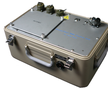
Battery-Powered Dart Control Unit
